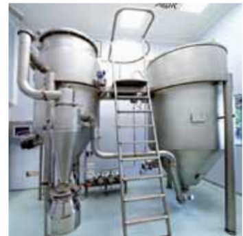
GEA Niro PHARMASD™ type PSD-2 spray dryer. Nominal drying gas rate: 360 kg/h.
