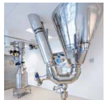
GMP suite with a GEA Niro PHARMASD™ type PSD-4 spray dryer in chamber with swing cone.
