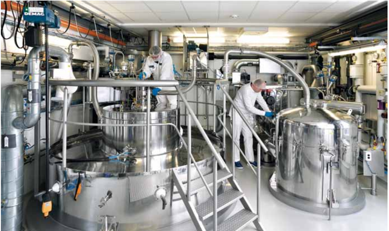
Custom-designed GEA Niro PHARMASD™ type PSD-4 chamber roof with gas disperser and top of bag filter.
