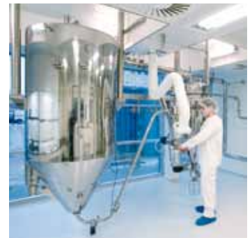
Custom-designed GEA Niro PHARMASD™ type PSD-1 spray dryer in clean room.
