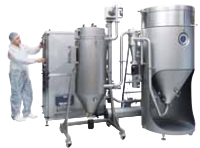
Standard GEA Niro PHARMASD™ type PSD-1 spray dryer for closed-cycle operation with solvent-based feeds. Nominal gas drying rate: 80 kg/h.
