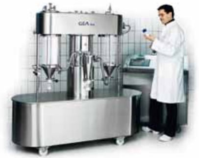
GEA Niro SDMicro™ R&D and laboratory spray dryer. Nominal drying gas rate: 30 kg/h.
