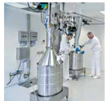
Powder collection in clean room, GEA Niro PHARMASD™ type PSD-4.
